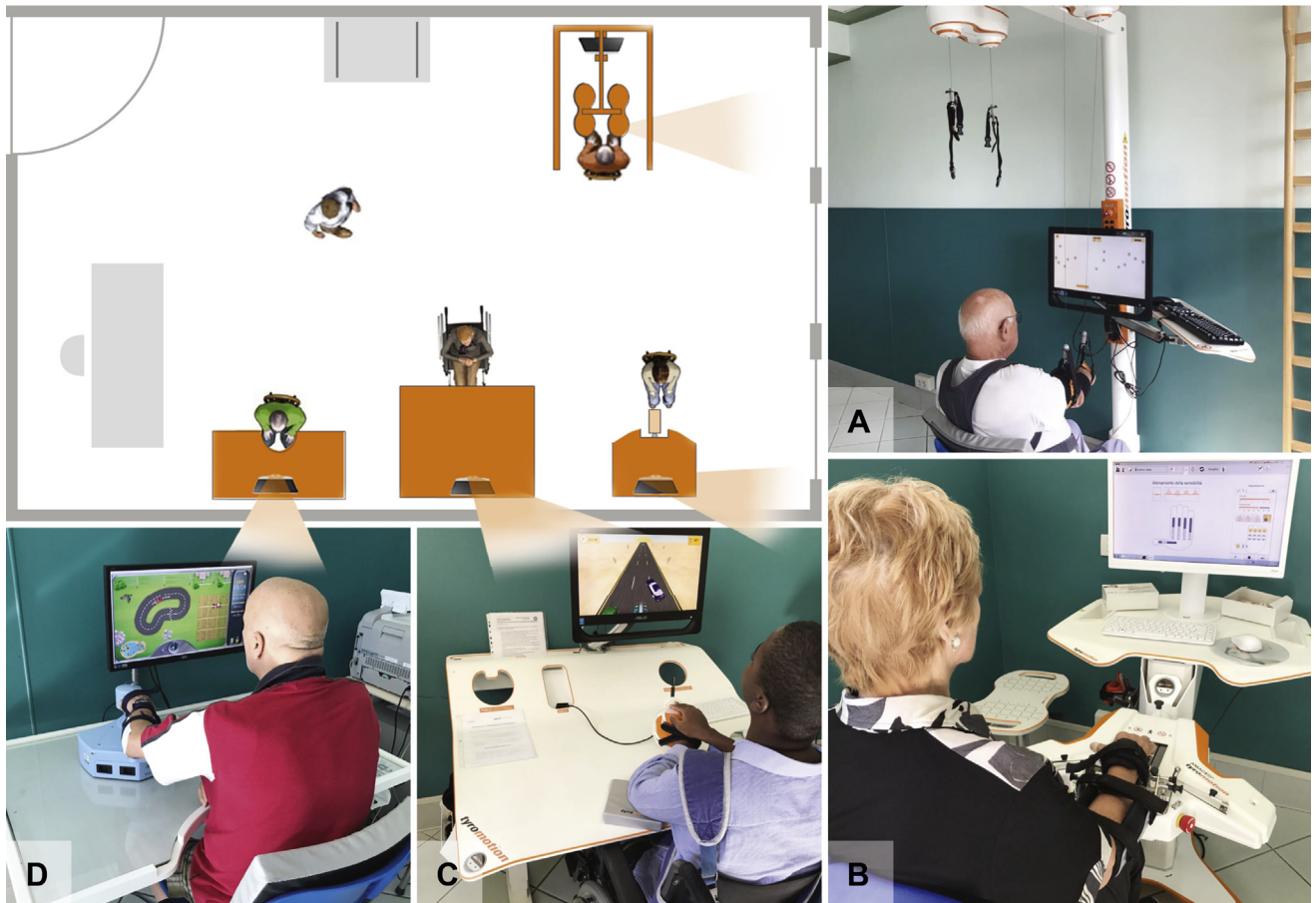
Figure 3. The Fondazione Don Carlo Gnocchi identified a set of 4 robotic and sensor-based devices to globally treat the upper limb: (A) a robotic arm-shoulder therapy system (DIEGO; Tyromotion), (B) a robotic finger-hand therapy system (AMADEO; Tyromotion), (C) a sensor-based therapy system for the entire upper limb (PABLO; Tyromotion), and (D) a robotic system for planar movements (Motore; Humanware).
